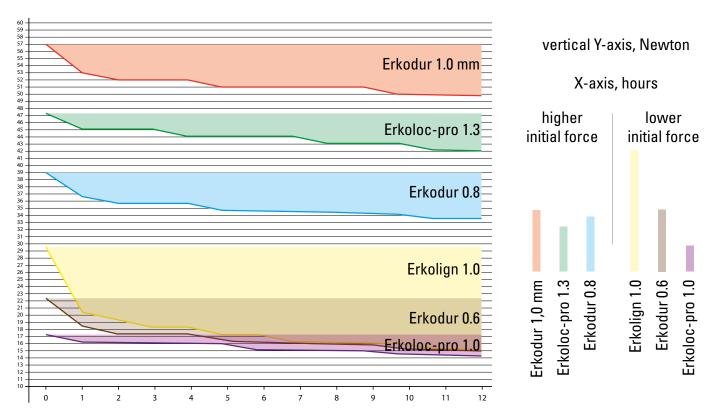
Conclusion: Laminated materials (Erkoloc-pro) have more restoring force respectively memory. That is, the corrective force is maintained for longer.
